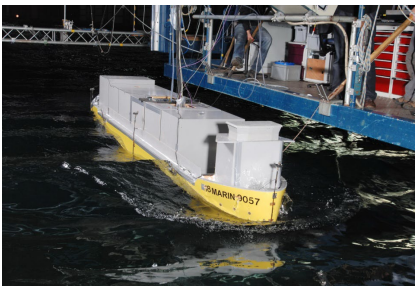
Model tests of an estuary ship in waves
